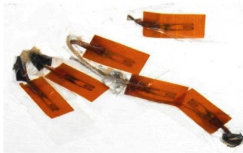
Figure 4. Type K ( CHROMEGA ®-ALOMEGA ®) thermocouples setup simulating the cardiac conduction system
