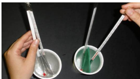
Figure 6. Measuring the time dependence of the temperature in both halves of a polystyrene glass with hot and cold water where the barrier is made of a conductor (left) and isolator (right). The experiment shows that the cold compartment absorbs approximately the same amount of heat that is released by the hot compartment.
