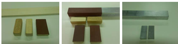
Figure 3. Surfaces proposed in the inquiry-based exploration on sliding friction: wood, sandpaper and steel.
