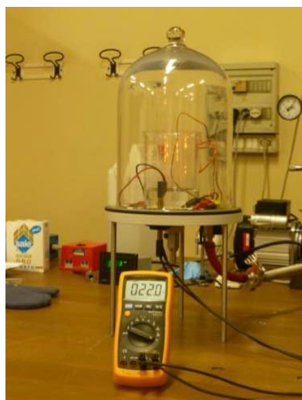
Figure 5. Experimental setup for the observation of phase transitions of water
