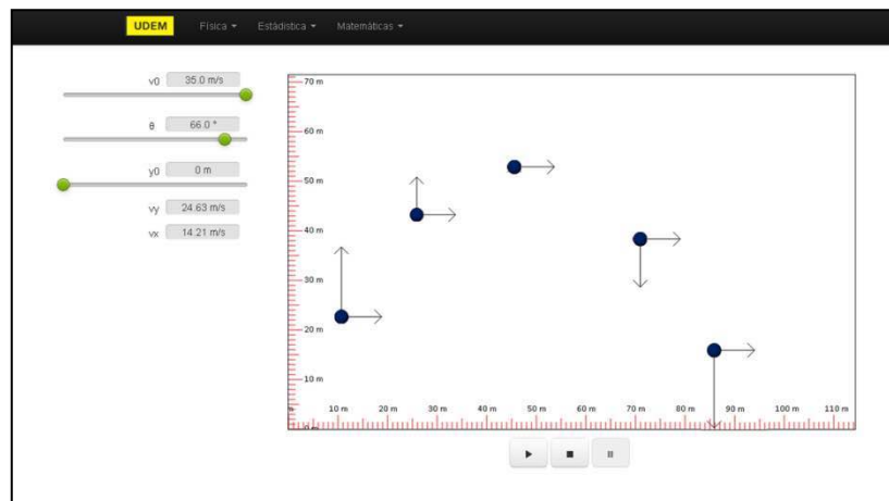
Figure 1. Computer simulation of parabolic projectile motion for using an initial velocity v_0=35 m/s and an angle \theta=66^\circ respect to the horizontal axis. The horizontal and vertical components at different times are shown to illustrate the difference between vertical (accelerated) and horizontal (constant) motion. The image is superimposed to show the evolution of the movement.
