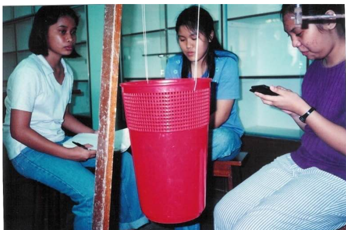
Figure 2: Rotation pendulum in the Philippines. Weights could be placed closer or farther from the center, strings could be
