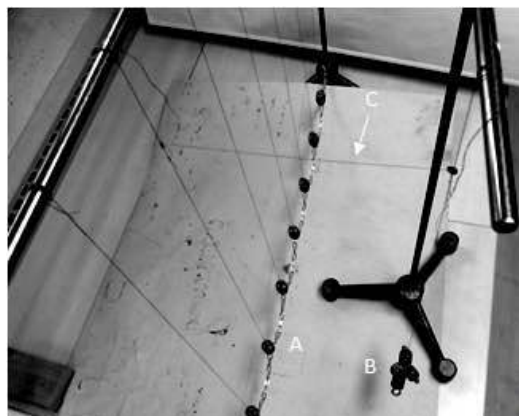
Figure 5. Coupled pendula can be used as a type of braced medium. The medium is made of pendula on strings coupled by a chain hanging from one pendulum to the next (A). On the bottom right side is the driving pendulum (B). A string (C) connects the string of the driving pendulum and one of the strings of the medium, and serves as coupling.
