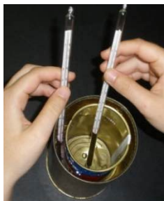
Figure 5. Measuring the time dependence of the temperature in cans with hot and cold water.
