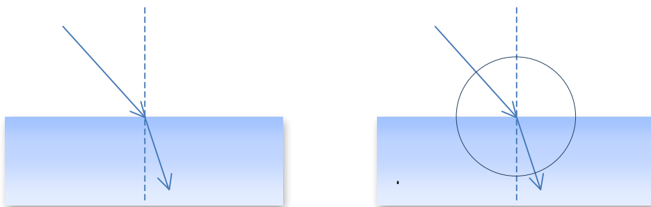
Figure 19. A geometrical construction of Snell's law
