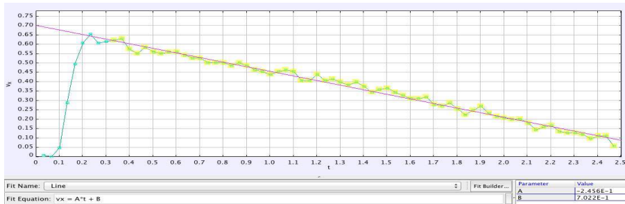
Figure 4. Tracker DataTool showing a Fit Line of v_x = -0.2456*t + 0.7022 .
