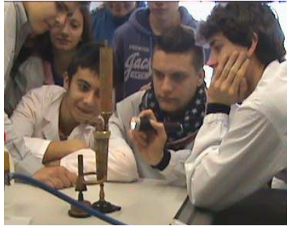
Figure 1. Students during the measurement of the alcoholic strenght of a solution by using the Malligand ebulliometer.
