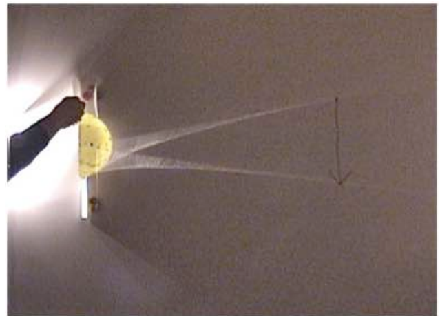
Figure 11. Apparatus in Figure 10 with both bulbs lighted, and the top half of the lens blocked by a card. Compare to Figure 3.
